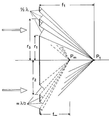
Fig. 3: Geometry of the zone plate.
