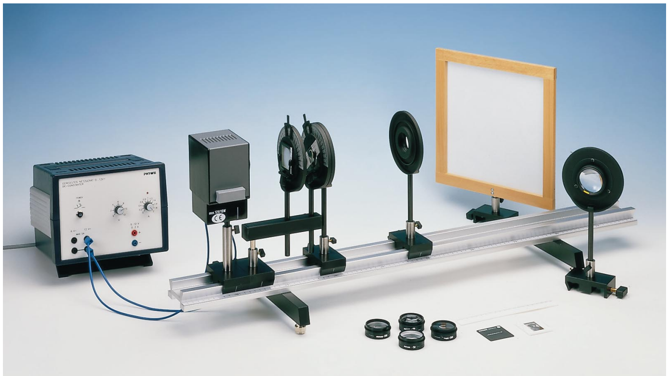
Fig. 1: Experimental set-up (microscope).
