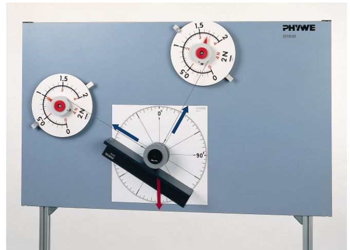
Resolution of forces on an inclined plane (MT 1.10)
