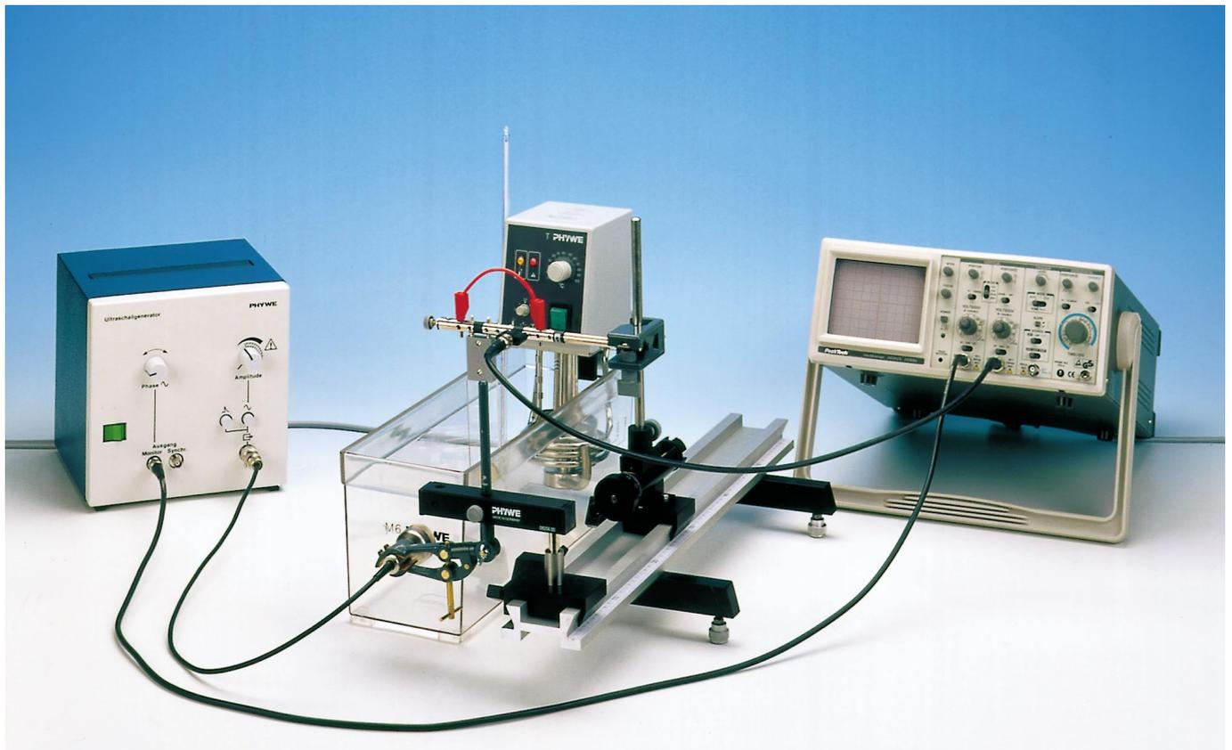
generator output. The pickup and monitoring signals are set in phase on the screen by moving the sound pickup and adjusting the phase control on the generator. The sound pickup is moved from this starting position and the wavelength is determined from the distance  $\Delta l$  through which it has been moved and the number  $n$  of inphase transition points traversed in the process.
