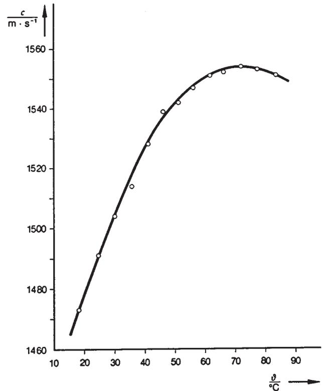
In Figs. 2 and 3 the velocities of sound found for water and glycerol in accordance with Eq. (4) and (5) are represented as a function of the liquid temperature.
