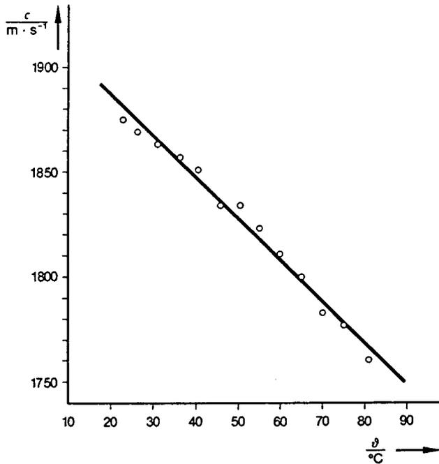
Velocities of sound with temperature coefficient
