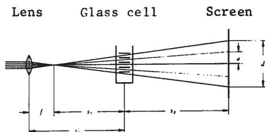
Fig. 3: Path of the rays in the central projection.
