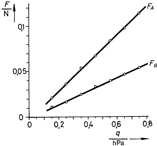
Fig. 3: Drag and lift in relation to the plate area for an angle of incidence of 20° and a dynamic pressure of 0.35 hPa.
