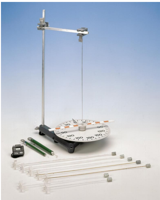
Fig.1: Experimental set-up for determining the torsion modulus of various bars.
