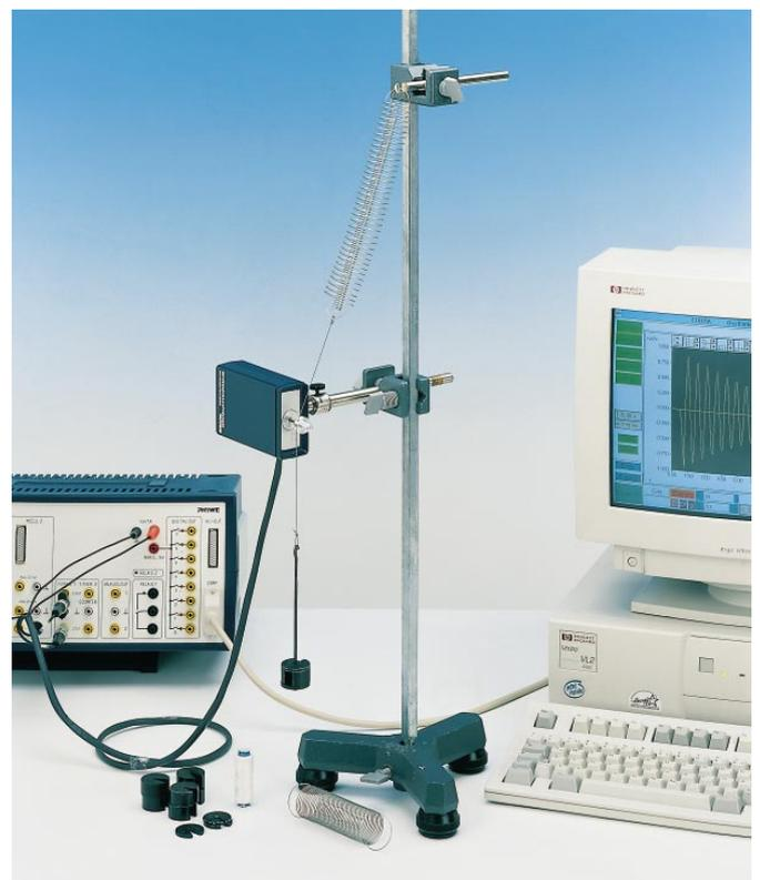
Fig. 3: Experimental set up for springs linked in series and in parallel.
