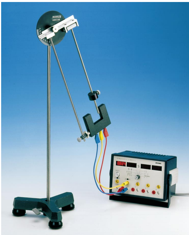
Fig. 1: Experimental set-up: Variable “g” pendulum.
