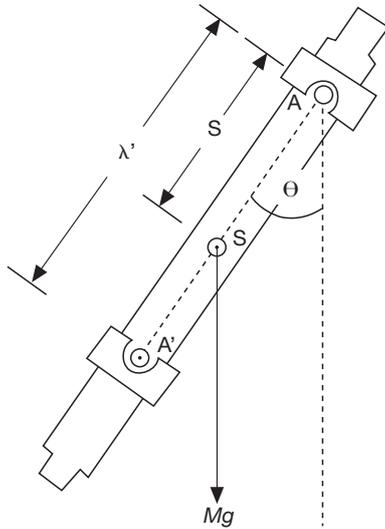
$$T_{kin} = \frac{\dot{\Theta}^2}{2} \sum_i m_i r_i^2 = \frac{1}{2} \dot{\Theta}^2 J = \frac{1}{2} \dot{\Theta}^2 (J_s + Ms^2) \quad (3)$$
