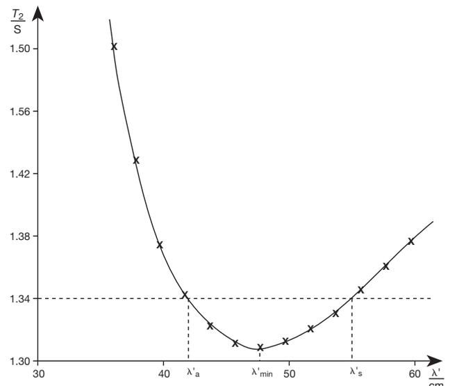
Fig. 3: Period  $T_2$  as a function of the position of the axis of rotation of the physical pendulum.
