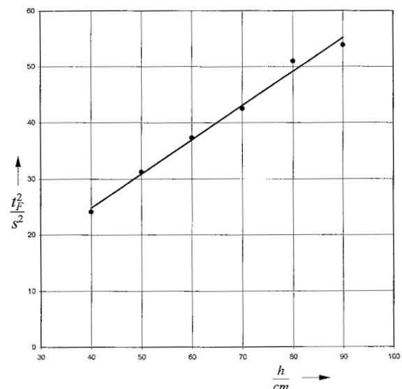
Fig. 3: Determination of the momentum of inertia from the slope of straight line  $t_F^2 = f(h)$ .
