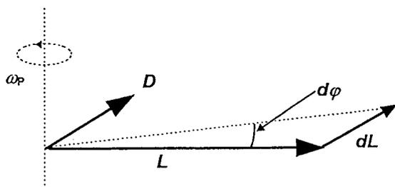
Fig. 5: precession of the horizontal axis of the gyroscope.
