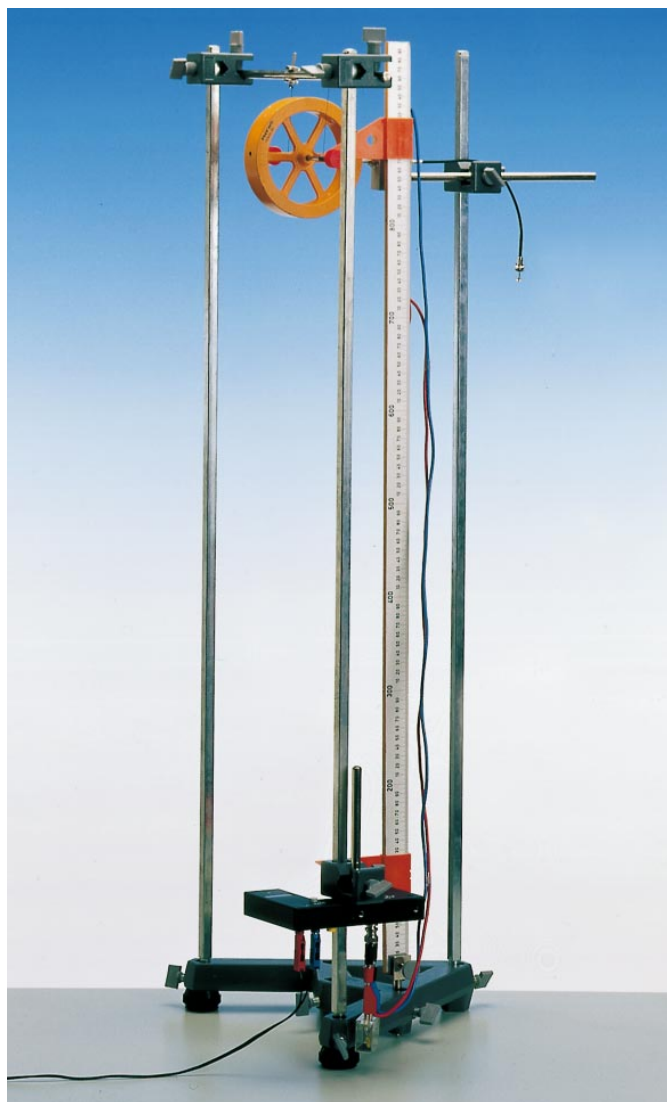
Fig.1: Experimental set up for investigating the conservation of energy, using the Maxwell disk.
