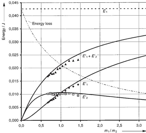
In an inelastic collision, only the momentum is conserved. In addition, the velocities after the collision are equal:
