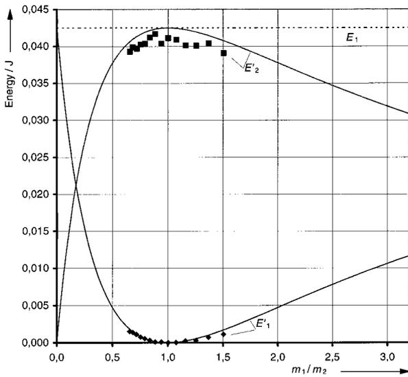
Fig. 7: Inelastic collision: energy after the collision as functions of the mass ratio of the gliders.
