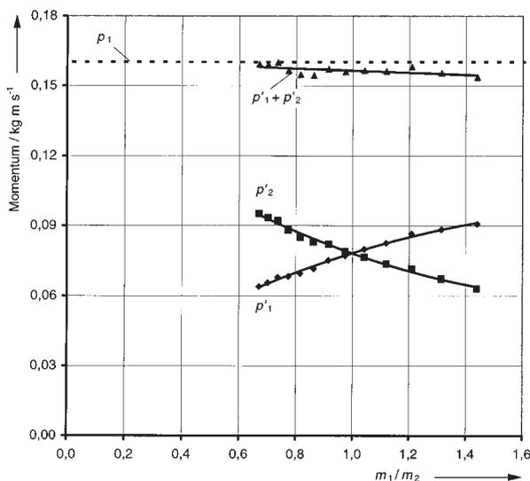
Fig. 6: Inelastic collision: momenta after the collision as functions of the mass ratio for the gliders.
