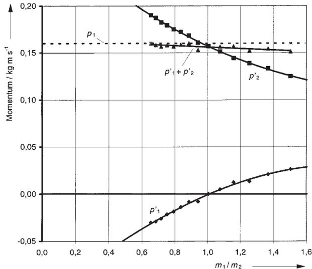
Fig. 4: Elastic collision: calculated momenta after the collision as functions of the mass ratio of the gliders.
