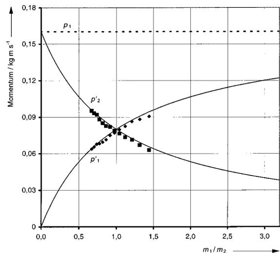
Fig. 8: Inelastic collision: calculated momenta after the collision as functions of the mass ratio of the gliders.
