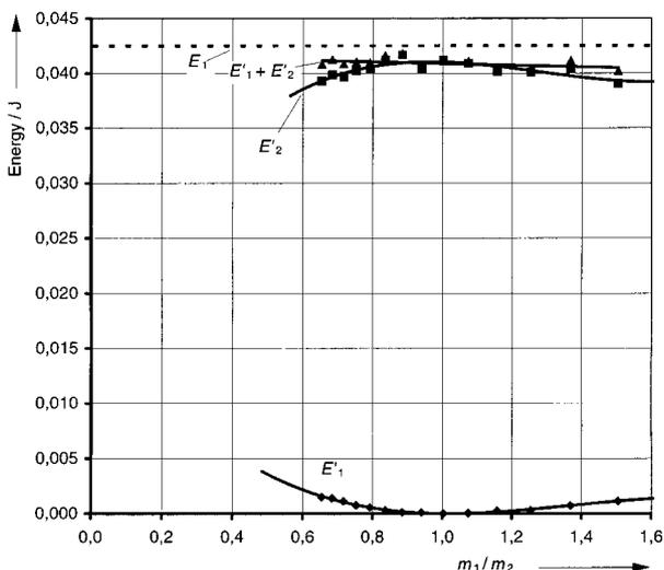
Fig. 3: Elastic collision: energy after the collision as functions of the mass ratio of the gliders.
