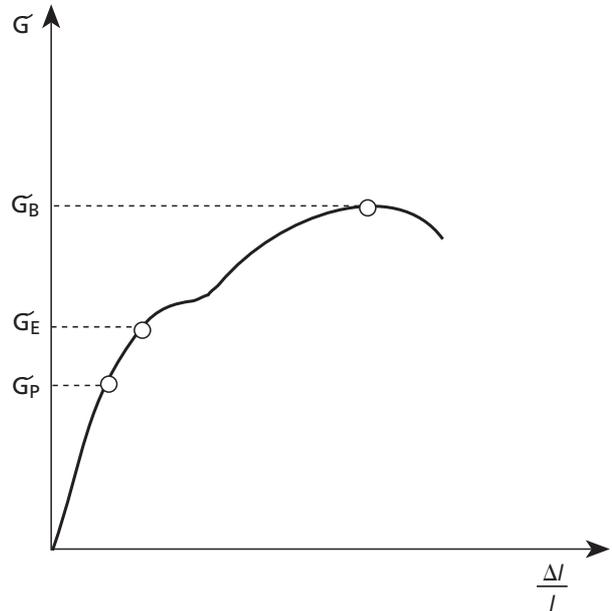
elongation  $\Delta l$  is no longer linear: elongation is larger than expected according to Hooke's law, considering the measurement values for small stresses (dotted line).
