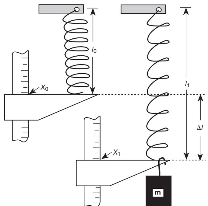
Fig. 3: Measurement of the elongation of the helical spring.
