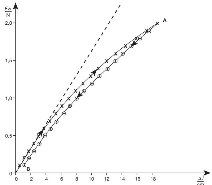
Fig. 7: Acting weight  $F_w$  as a function of the extension  $\Delta l$  for a rubber band (elastic hysteresis).
