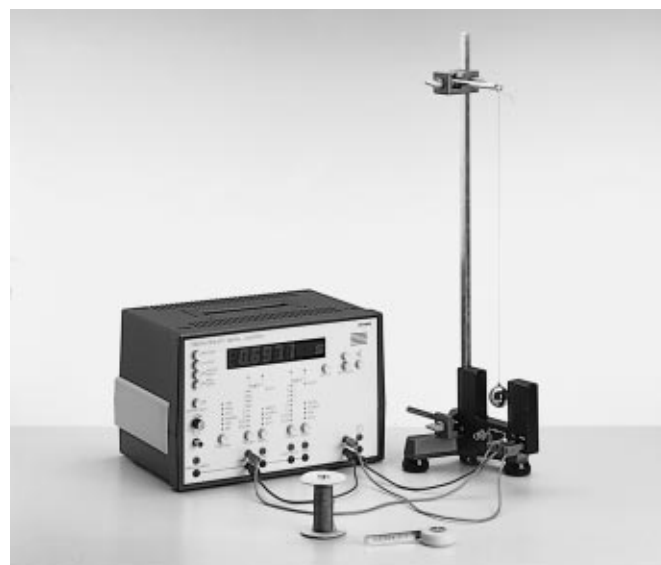
Fig. 6: Experimental setup: Frequency measurement of a pendulum. (In Fig. 1 the alternative with the 4-decade counter is shown).
