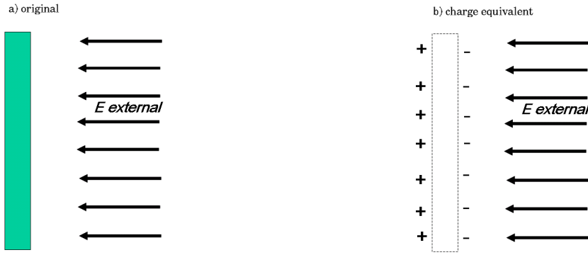
Figure 1.30: a) An infinitely large conducting plate is placed in an external electrical field in the z direction. b) The physical equivalent charge configuration on the plate.
