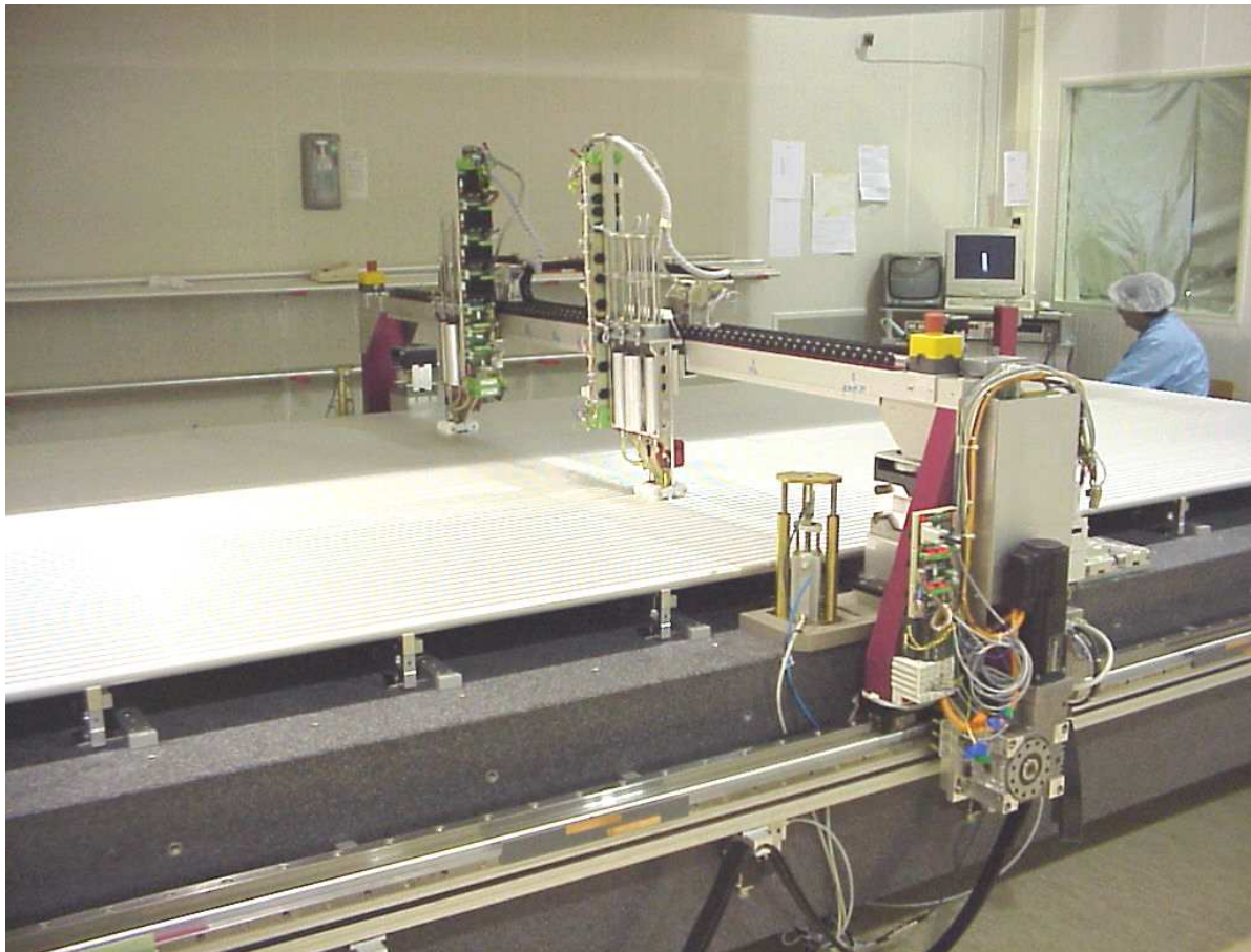
Figure 11: Glue is dispensed on a tube layer by the gluing machine.
