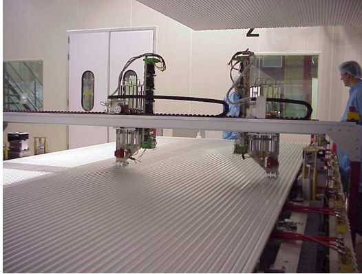
Figure 19: a) Glue dispersion by the gluing machine. b) attaching another layer.
