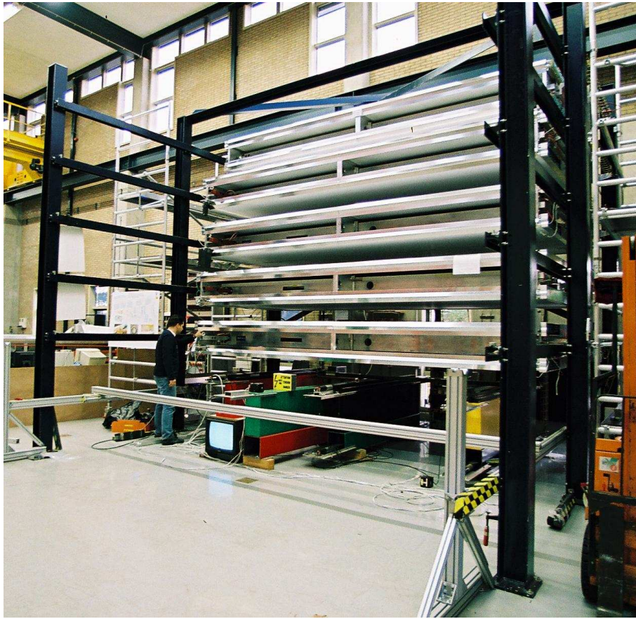
Figure 24: Picture of the NIKHEF cosmic ray test facility with five BOL chambers. The chamber in the highest position is - in this particular case - a small type BOL chamber with a width of 48 tubes, the others are standard BOL chambers.
