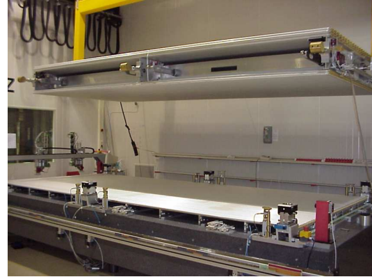
Figure 19: a) Glue dispersion by the gluing machine. b) attaching another layer.
