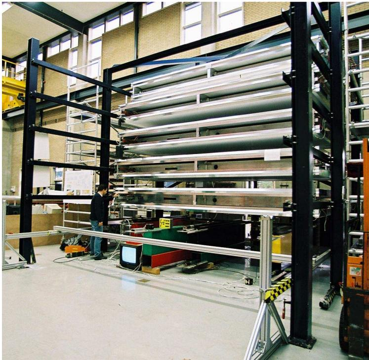
Figure 25: Picture of the cosmic ray stand with five BOL chambers. The chamber in the in the highest position is a small type BOL chamber with a width of 48 tubes.
