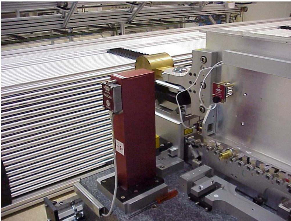
Figure 15: The picture shows the stacking tower supporting the extension of the spacer. The position of the spacer is monitored the alignment system. xxxxxxxxindicate in the piture?xxxxxxx
