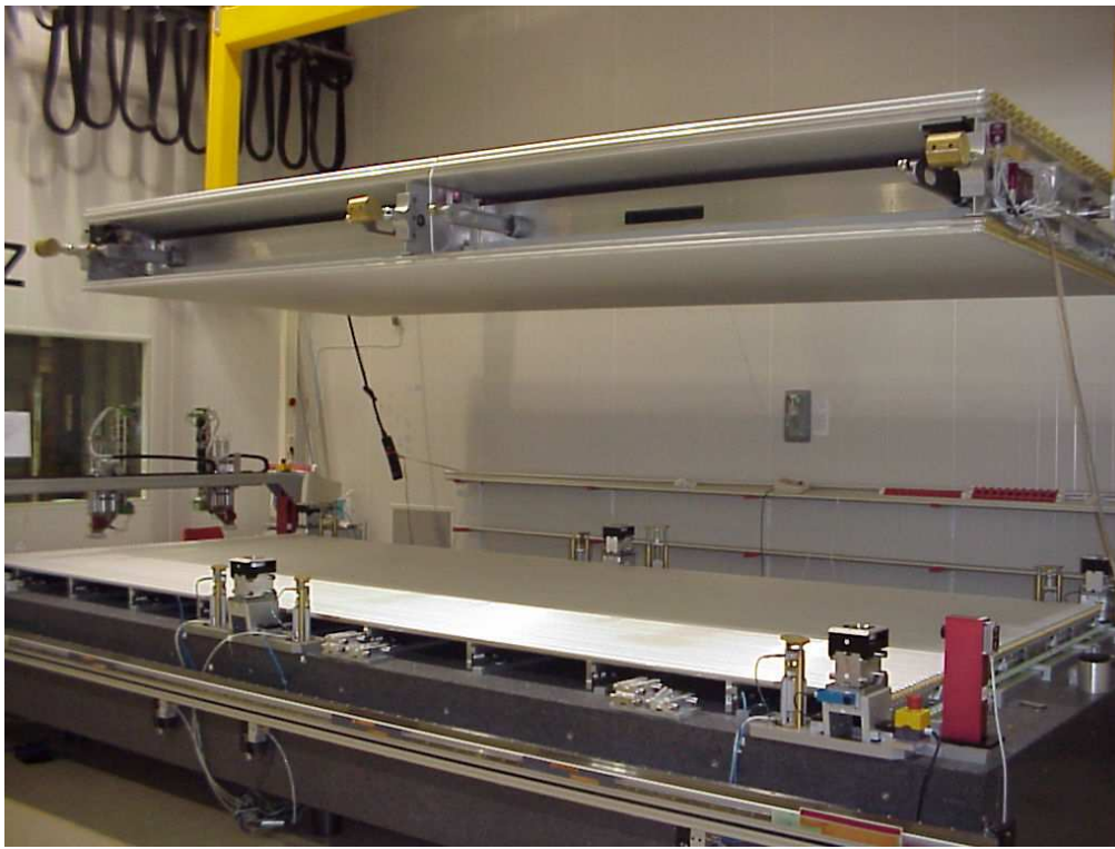
Figure 14: Picture taken in the cleanroom, illustrating the last step of the chamber assembly. The jigs on the granite table hold the final tube layer. The chamber, which consistst at this point of the spacer with 3 layers on top and 2 layers at the bottom is lowered on the last tube layer. Also visible are the stacking towers, sag compensation towers and RASNIK towers that control the positioning of the spacer. (xxxxxxxxxx indicate this in pixture? xxxxxxxxx)
