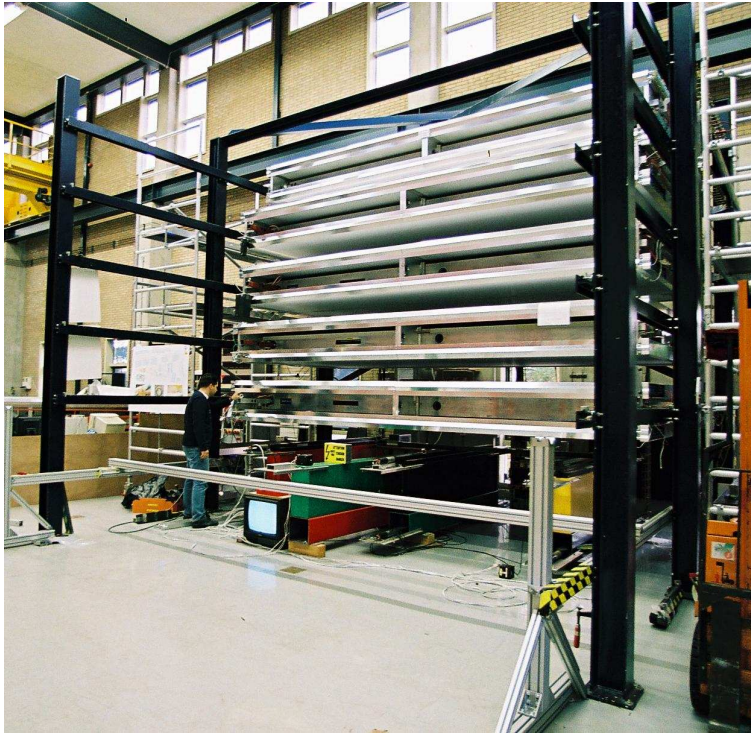
Figure 21: Picture of the cosmic ray stand with five BOL chambers. The chamber in the in the highest position is a small type BOL chamber with a width of 48 tubes.
