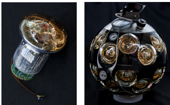
Figure S.3: Left: A KM3NeT photo multiplier tube (PMT).
