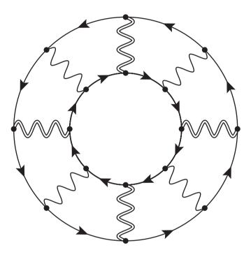
The double wiggles are W-bosons (with V-A coupling) and the normal wiggles are photons. Try to work out this trace in 4 dimensions (forget about the denominators). Hint: use  $\infty_{7}$ . Assume that photons do not change the mass of a particle, but W-bosons do
