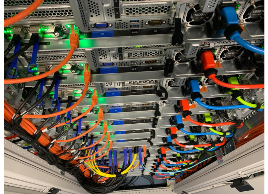
Image: Cluster ‘Lotenfeest’ at the Nikhef NDFP, acquired March 2020. Lenovo SR655 with AMD EPYC 7702P 64-Core single-socket
