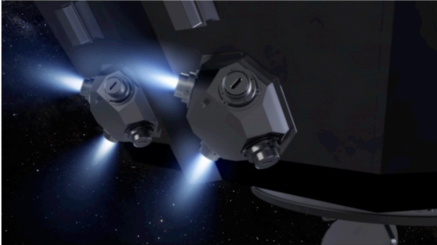
Microthrusters will make minuscule shifts in order to keep the spacecraft centered on one of the masses. This will isolate the two cubes from all external and internal forces except gravity, placing them in the most precise freefall ever obtained.
