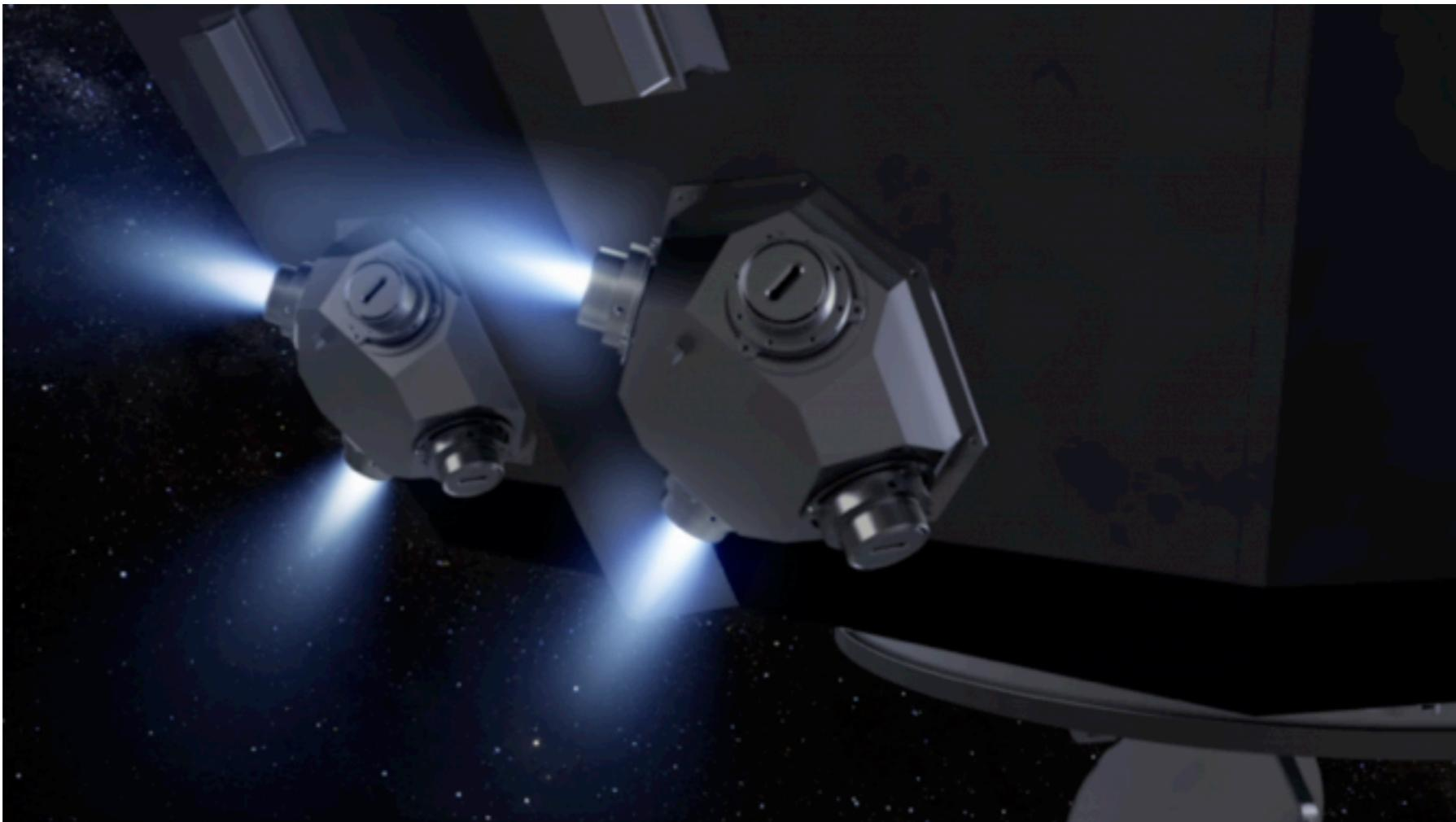
Microthrusters will make minuscule shifts in order to keep the spacecraft centered on one of the masses. This will isolate the two cubes from all external and internal forces except gravity, placing them in the most precise freefall ever obtained.
