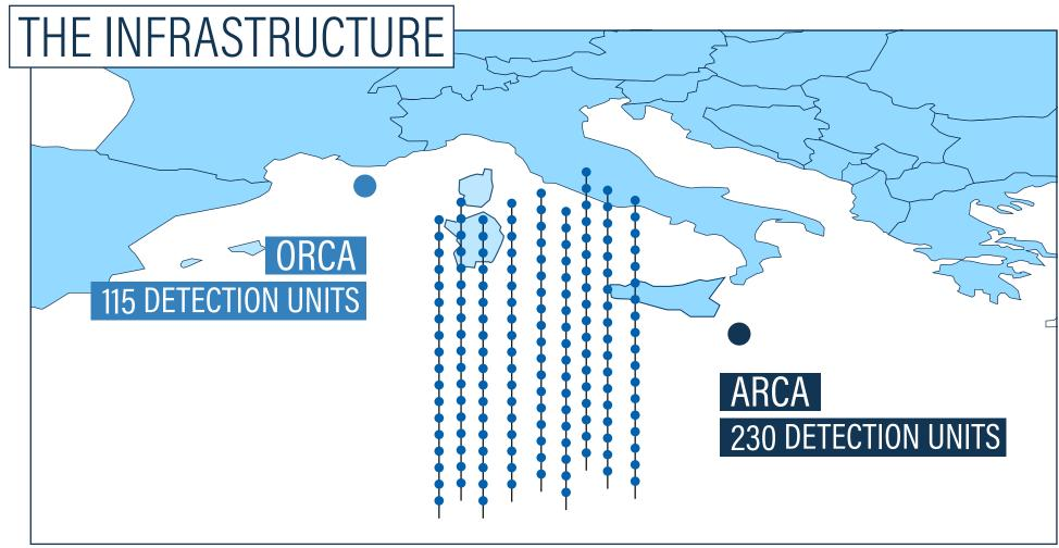
The KM3NeT infrastructure consists of an array of hundreds of detection lines, "detection units", which stand on the sea bottom and are equipped with thousands of hi-tech eyes. Its final configuration will occupy a volume of over 1 km<sup>3</sup>, hence its name.
