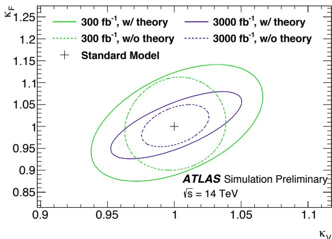
Figure S.2: 68% CL expected likelihood contour for  $\kappa_V$  and  $\kappa_f$  in a minimal coupling fit at 14 TeV for an assumed integrated luminosity of  $300 \text{ fb}^{-1}$  and  $3000 \text{ fb}^{-1}$ .
