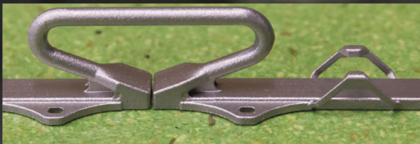
Figure 4. Lara Veldt shows two connected 3D-printed, 0.2 mm wall thickness multichannel titanium cooling-structures, to be mounted inside the read-out box of the scintillation fiber tracking detector of the LHCb upgrade.
