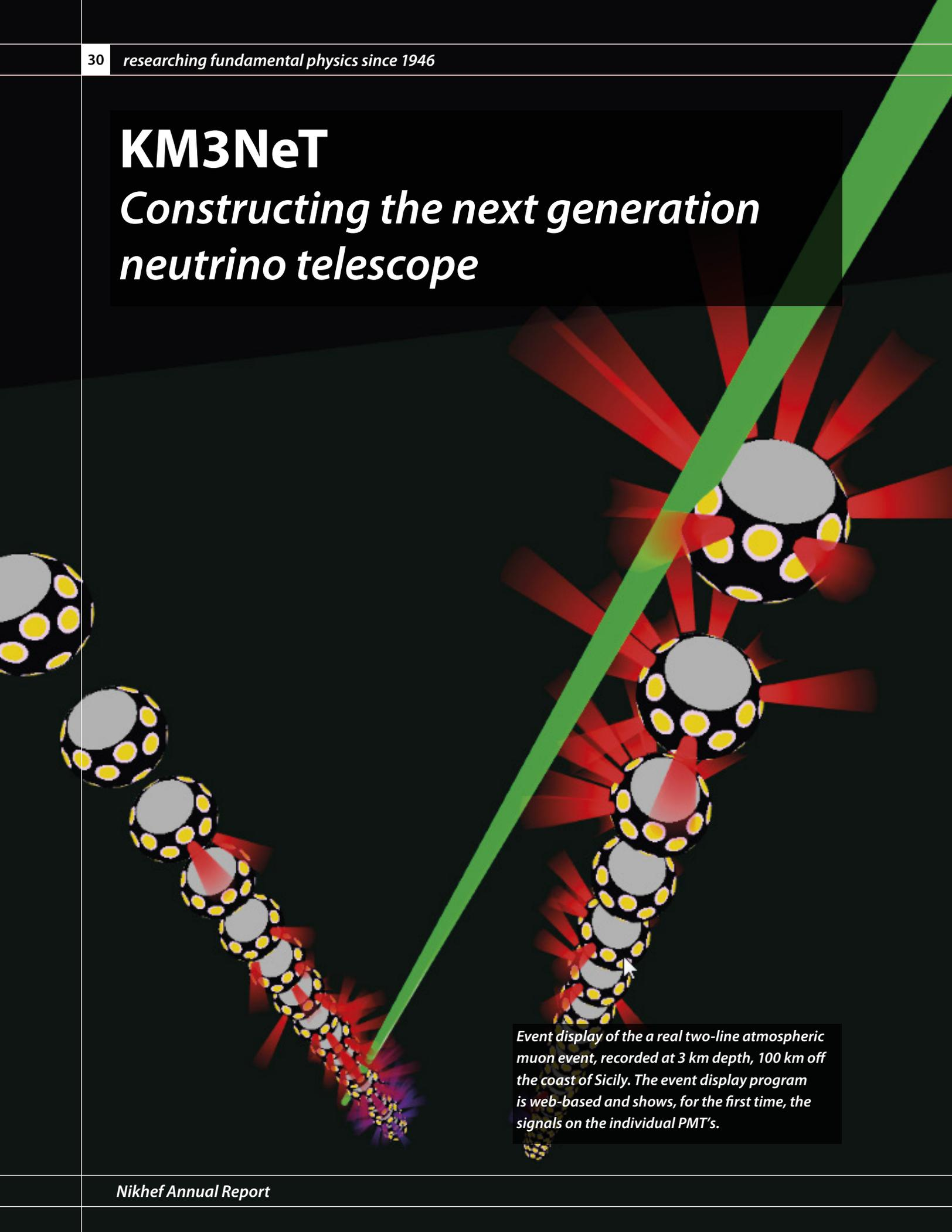
*Event display of the a real two-line atmospheric muon event, recorded at 3 km depth, 100 km off the coast of Sicily. The event display program is web-based and shows, for the first time, the signals on the individual PMT's.*
