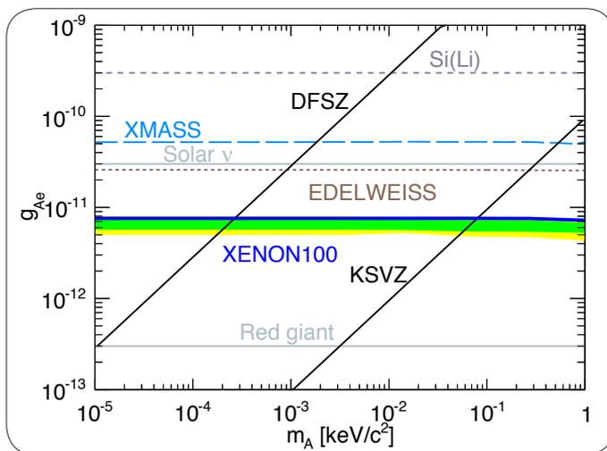
Figure 1. The XENON100 limit (90% CL) on the axion-electron coupling constant vs solar axion mass (blue line). The expected sensitivity is shown by the green/yellow bands ( $1\sigma/2\sigma$ ). Two benchmark axion models, DFSZ and KSVZ, are represented by grey lines. Within these models, XENON100 excludes axion masses above  $0.3 \text{ eV}/c^2$  and  $80 \text{ eV}/c^2$ , respectively.
