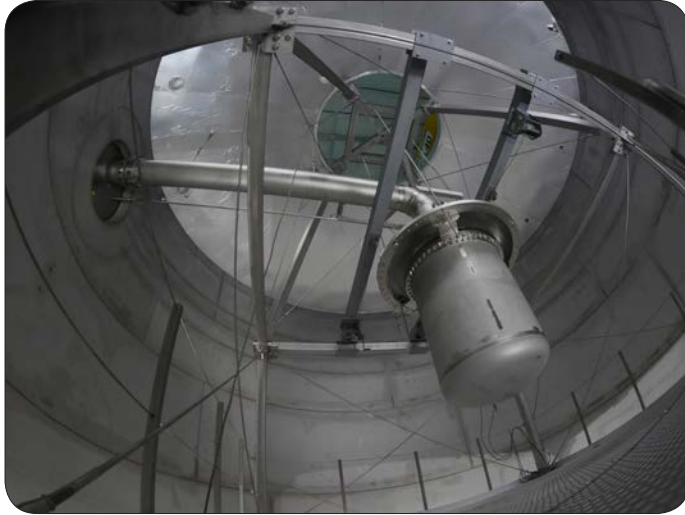
Figure 2. View of XENON1T inside the water Cherenkov muon veto. The inner cryostat vessel, which will house the TPC, is hanging from the cryostat support structure. The large pipe will carry all the cryogen and signal lines from the cryostat to the support building outside of the water tank.
