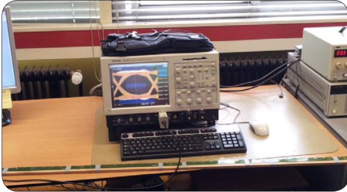
Figure 2. Test set-up for signal transmission tests
