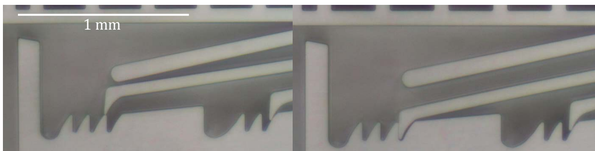
Figure 47. Locking of the Shuttle in the 5 th Shuttle lock. Left: the final position of the Shuttle hooks of the quasi-static measurement shown in figure 46. Right: the Shuttle hook is locked in the 5 th Shuttle lock after a 25 ms pulse with U_{ETA} = 16,79 V.
