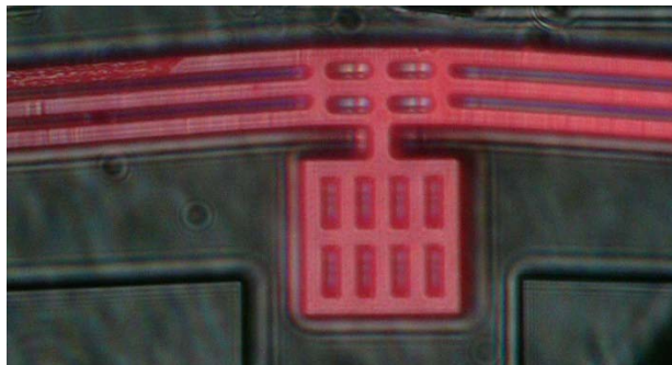
Figure 57. Red glowing of the Back ETA in vacuum at P_{ETA} = 186 \text{ mW} .
