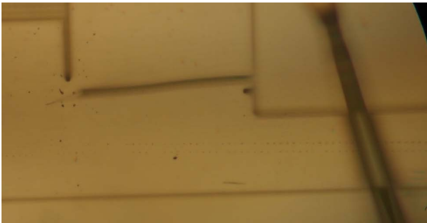
Figure 9: Dotted sacrificial layer remains below a destroyed ETA beam, with structure thickness of 6 \mu\text{m} . Also four spots are shown at the place of the fillets of a bi-stable beam structure. Focused on substrate, 200x magnification.
