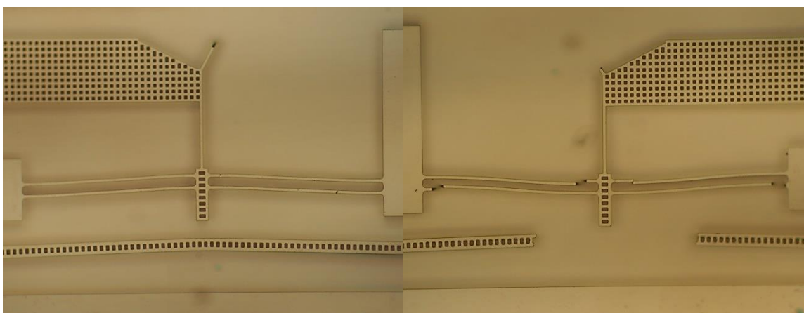
Figure 3: (a) Bi-stable beam successfully flipped by ETA. (b) Bi-stable beam and ETA broken by stress. It is still uncertain if the ETA beam or the bi-stable beam failed first and destroyed the other by impact. It is certain that the ETA beam was at its limit in this case, because it showed melting spots.
