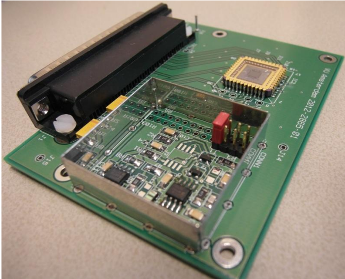
Figure 78: In-vacuum electronics chip board with soldered chip carrier.
