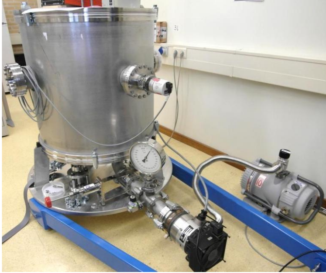
Figure 53: Vacuum chamber set-up. Evacuation by scroll pump and second stage turbomolecular pump.
