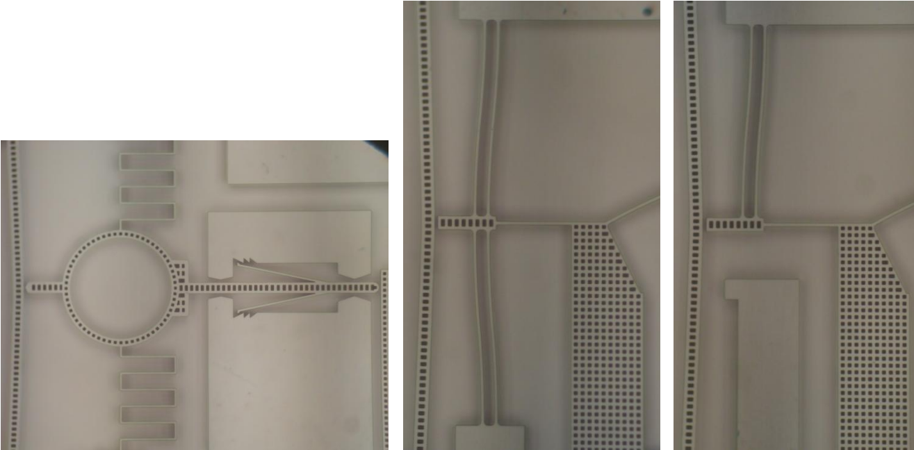
Figure 76: From left to right, G1 anti-reverse, G2 bi-stable, G3 single guiding. 200x magnification microscope.
