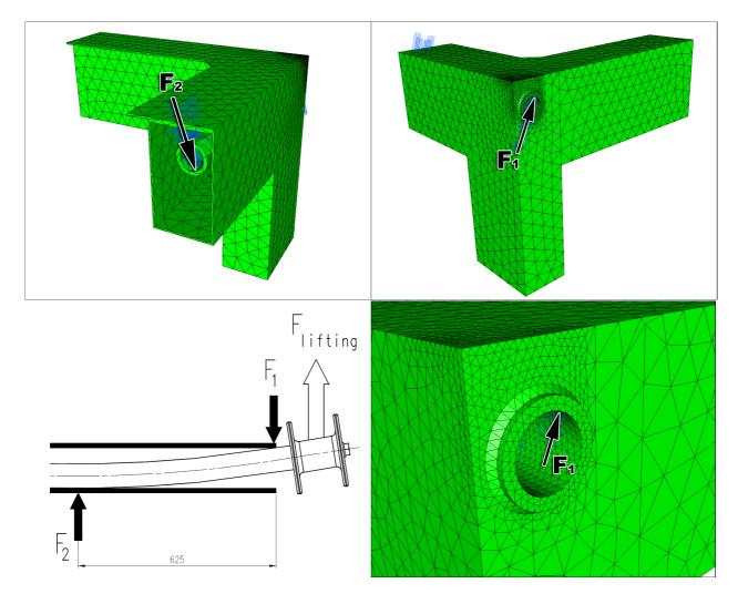
Mesh type(s): Load(s): 3D Solid parabolic tetrahedron
