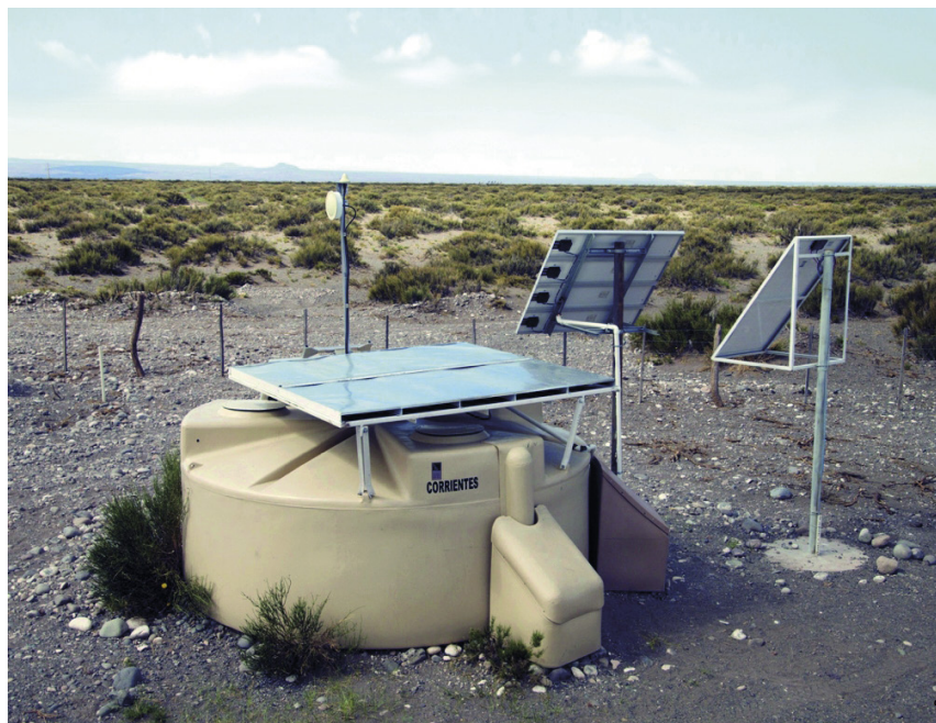
Figure 3. The scintillator surface detector (SSD) as seen on top of the Cherenkov tank. It consists of a 1 cm thin plane of nearly 4 m 2 of scintillator, read out by a single photomultiplier.
