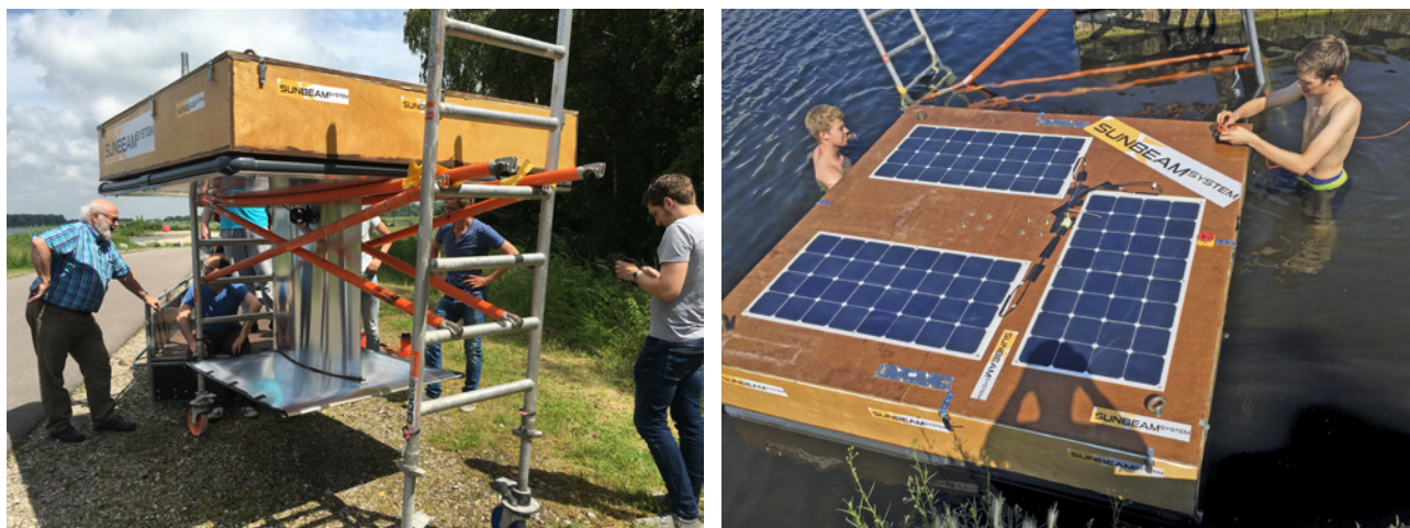
Figure 1. As part of the MSc course 'Nikhef project', students built an autonomous cosmic ray muon scintillator detector that was tested in the waters around Nikhef (Photo credit: Wesley Poland).
