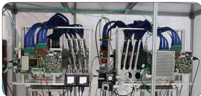
Figure 1. LHCb telescope with eight sensor planes bonded to Timepix3 front-end chips and read out by the SPIDR data acquisition system
