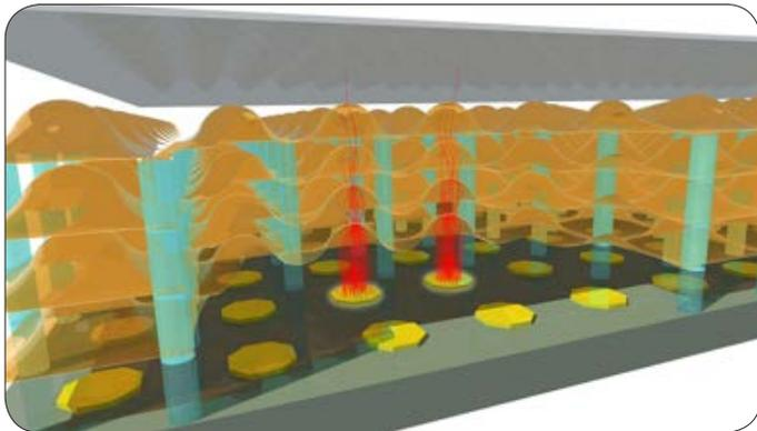
Figure 3. A stack of ultra-thin transmission dynodes forms a ‘miniaturised’ PMT on top of each  $55\ \mu\text{m}$  squared pixel of the readout chip at the bottom. A photoelectron escapes from the photo-cathode at the top, further electron multiplication results in a detectable signal that will be processed by the front-end circuitry in each pixel.
