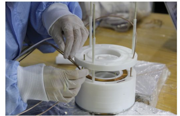
(b) Installation of a field-shaping ring..
