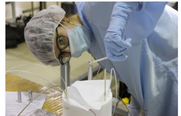
(f) Screwing together suspension assembly.
