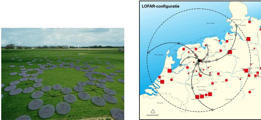
Fig. 10: The layout of the LOFAR radio telescope.
