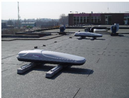
Fig. 9: Pair of HiSPARC scintillation detectors.
