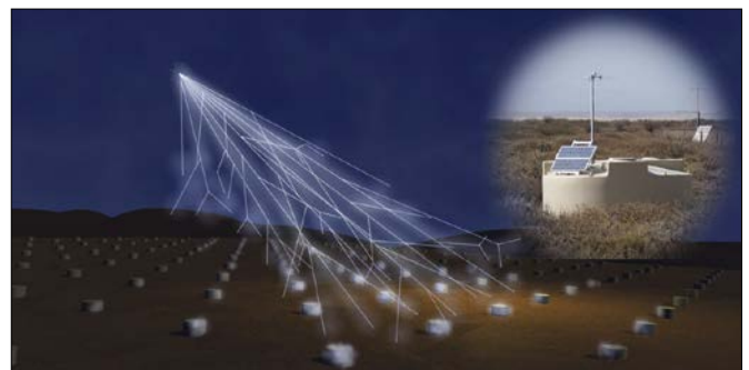
Figure 12. Artist's impression of a cosmic-ray shower development in air. The inset shows a Pierre Auger surface-detector station with a radio-detection station barely visible in the background.
