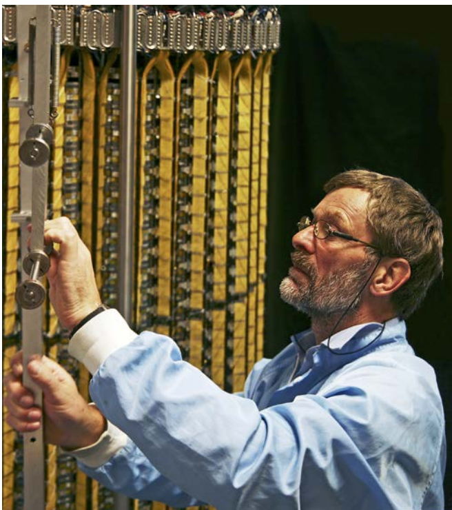
Figure 18. The ALICE Silicon Strip Detector during completion at Utrecht University.
