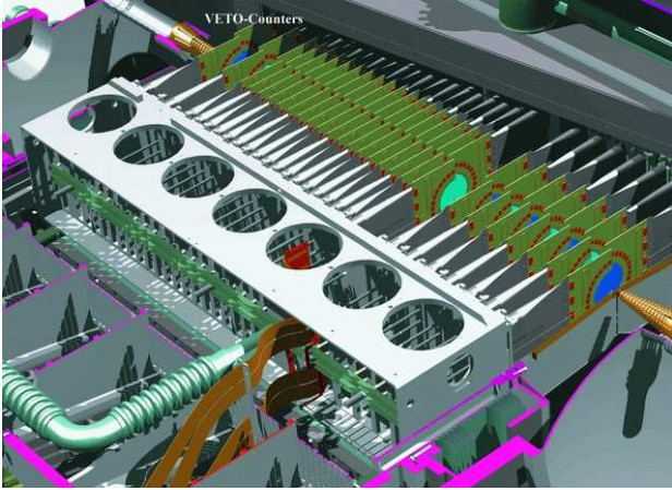
Figure 2: Layout of the Vertex tank with indicated the 2 planes of VETO detectors.
