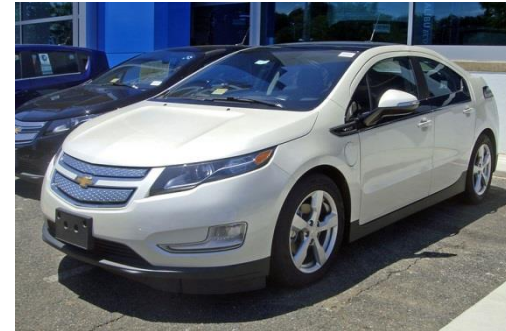
Volt/Ampera: Battery pack 16.5 kWh Tesla: 60 – 85 kWh
