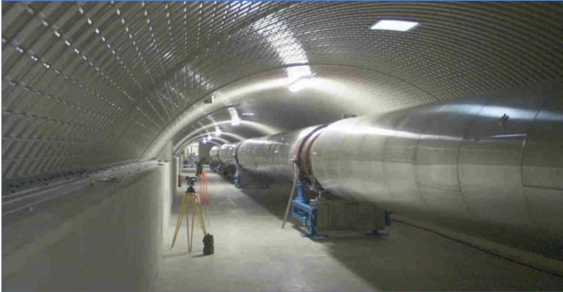
Largest vacuüm vessel in Europe: Pressure \sim 10^{-10} mbar
