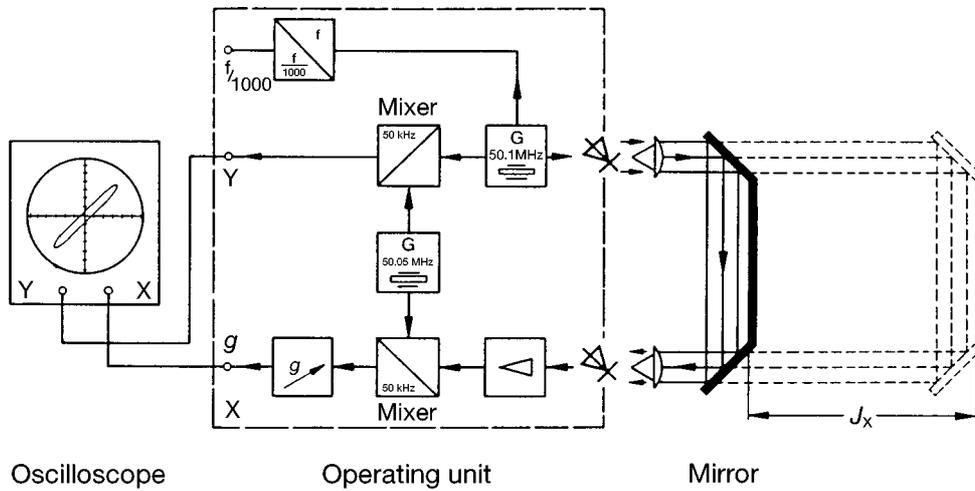
rays and the mirror moved until the Lissajous figure again shows the same phase difference.
