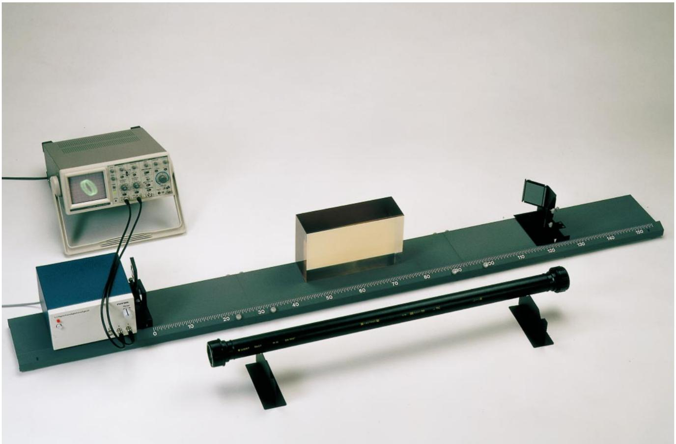
Fig. 2: Diagram of the experimental set-up for measuring the velocity of light in air.
