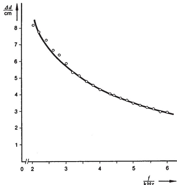
Fig. 3: Resonance wavelength dependent on the displacement  $\Delta d$ .
