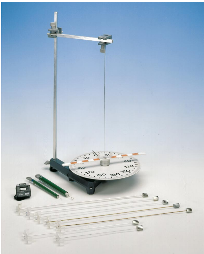
Fig. 1: Experimental set-up for measuring the hysteresis of metal bars in torsion.
