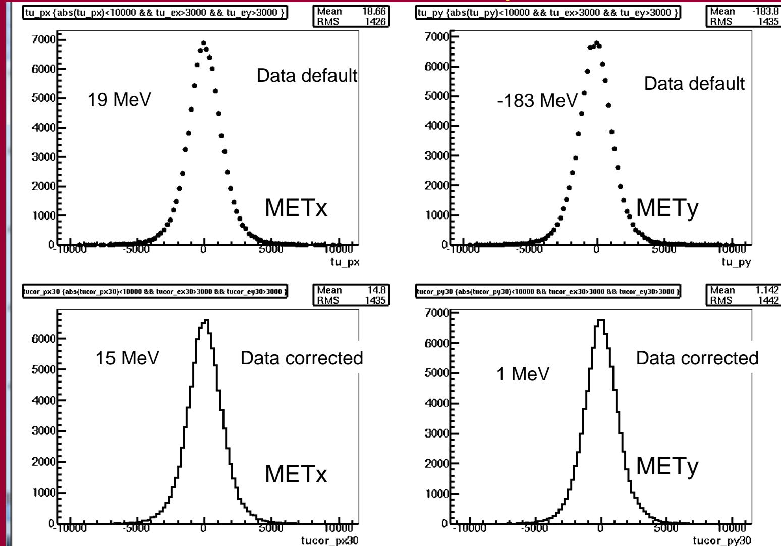
DATA corrected = Vtx correction + 2mm FCAL shift + R=105mm cut
