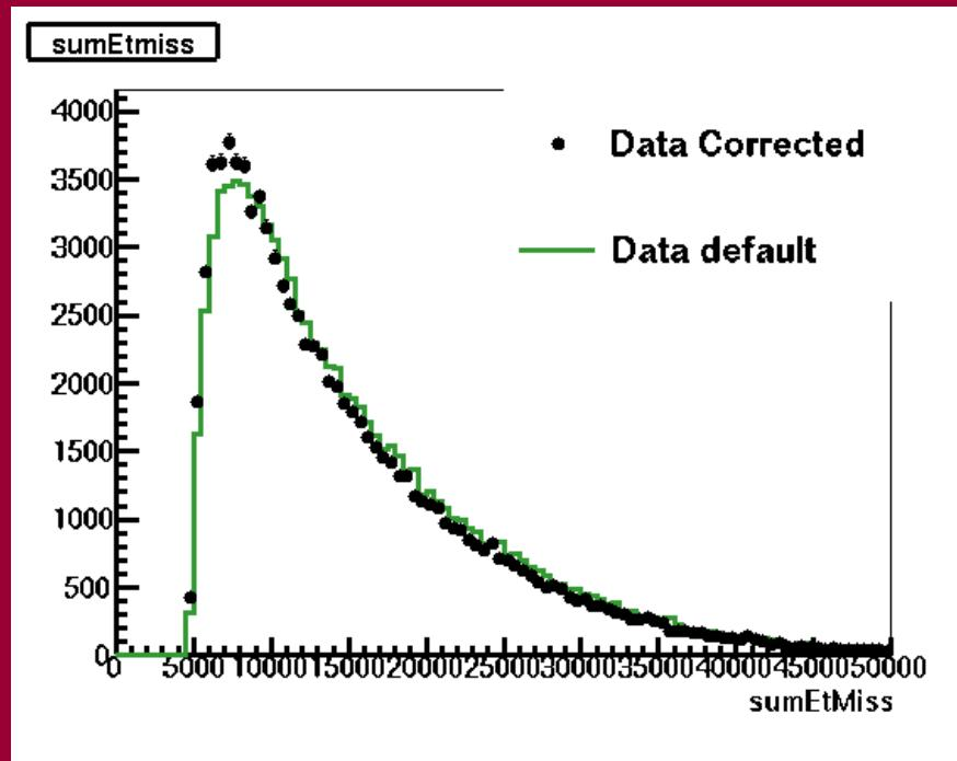
Data Corrected= Vtx correction + 2mm FCAL shift + R=105mm cut
