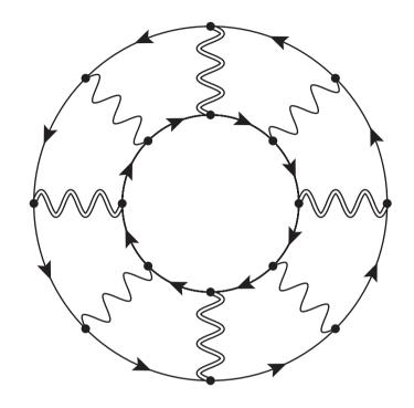
The double wiggles are W-bosons (with V-A coupling) and the normal wiggles are photons. Try to work out this trace in 4 dimensions.
