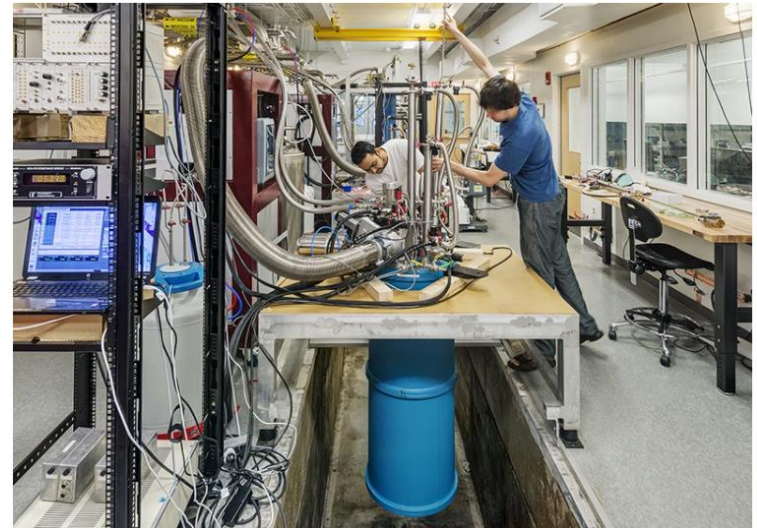
Experiments to find Majorana signals are performed by loading a nanowire into a dilution refrigerator capable of cooling it down to close to absolute zero. Credit: HGA Architects and Engineers
